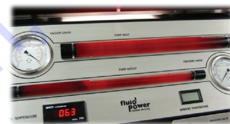
Transparent, back-lit suction and pressure lines
