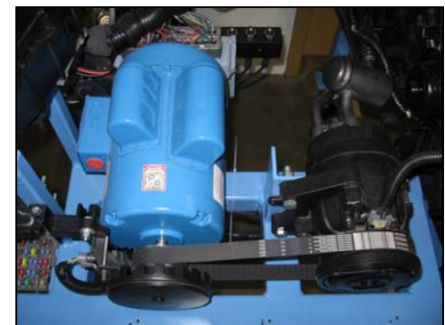
EM-101 ELECTRIC MOTOR AND VACUUM PUMP
