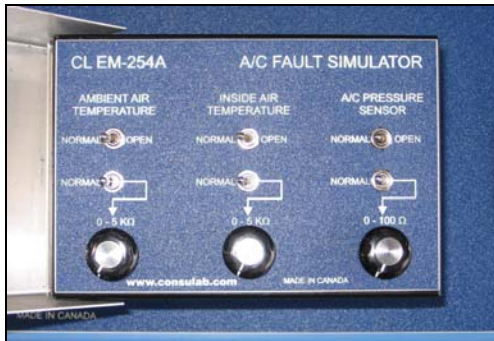
EM-254, LOCKABLE FAULT SIMULATOR FOR A/C
