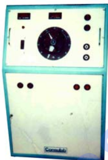
Model CL-7108D Bench for 0-12 V AC; 0-12 V DC
